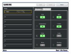
Note: Although you can configure stereo channels, Ganging is the preferred method for linking channels when mixing live. Creating and removing gangs can be carried out quickly 'on the fly' while mixing. However, configuring stereo channels using the MIXRACK SETUP / Mixer Config screen resets the DSP architecture, takes a while to complete, and should only be used for setting up 'permanent' stereo channels, for example walk-in music players and external effects returns.
